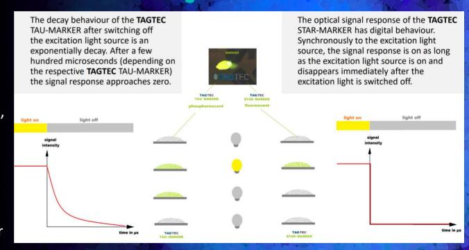
be in the UV, visible or NIR range. Detection takes place after the primary light source is switched off. The afterglow of the phosphorescent marker is evaluated using TAU determination.
